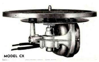
Model CX - Direct drive, self. starting induction type motor. Fan-cooled. Fully enclosed, with silent helical-cut gears running in oil bath in scaled housing. Double - insulated drive sleeve. Delivered ready to install. Choice of 8", 9", 10" or 12" turntable.
